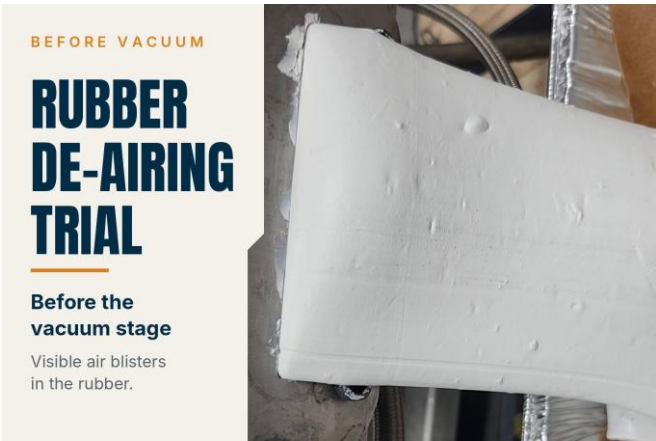
Before vacuum: feeder output with visible air blisters.
