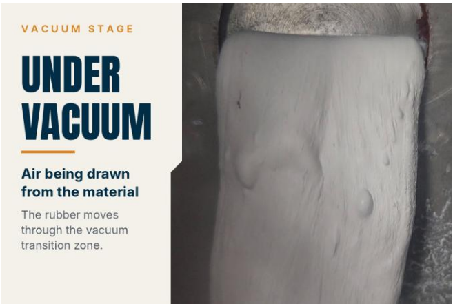
Vacuum section: blistered strip moving through the transition zone.
